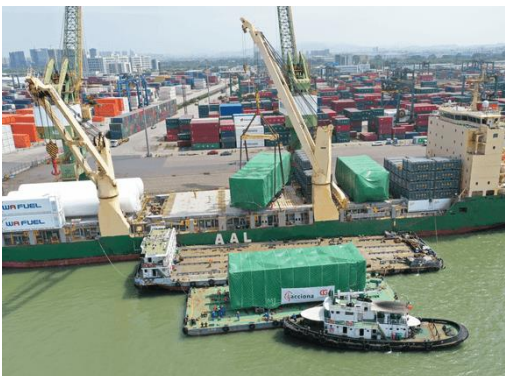
Singapore-headquartered AAL Shipping's multipurpose vessel AAL Nanjing being loaded with chimney sections in China for a mining facility in Australia. Photo credit: AAL Shipping
